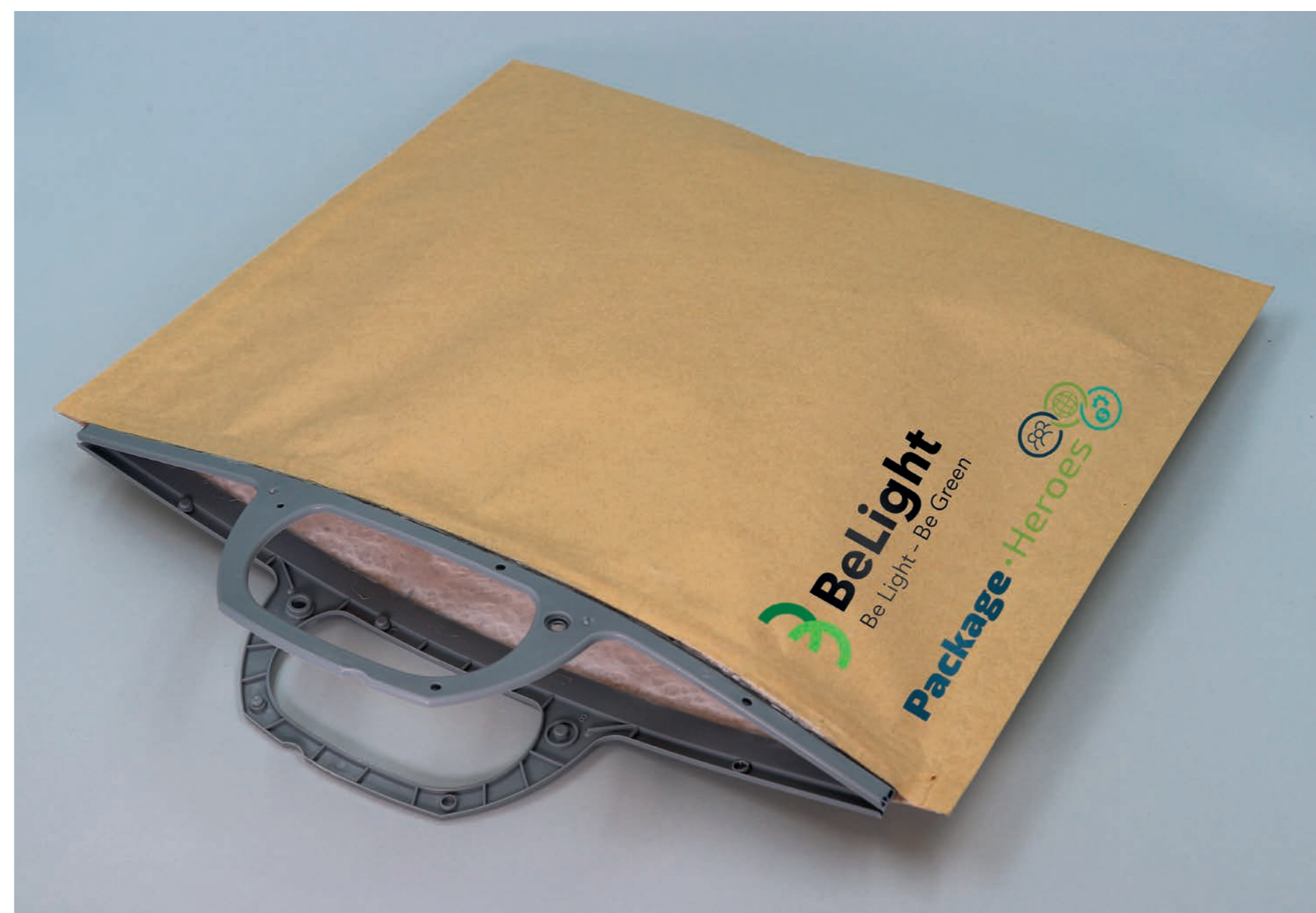
Figure 2: In the biopolymer based compostable thermal insulation bag demonstration, the thermal insulation is a thin extrusion foamed PBSA foam and film, and the cover is a PBSA coated kraft paper (the extrusion coating was performed in the Package Heroes –project). PBSA (Poly(butylene succinate-co-adipate)adibate)) is a bio-based, flexible and home compostable thermoplastic material.
