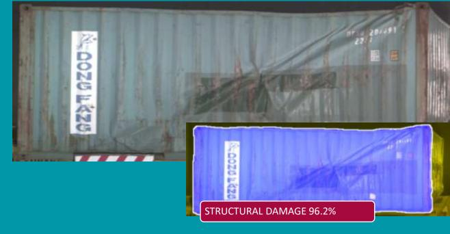
Automated detection of damages in cargo containers is a central part of asset management.
