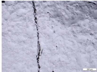
A "fresh" scratch on the coating surface
